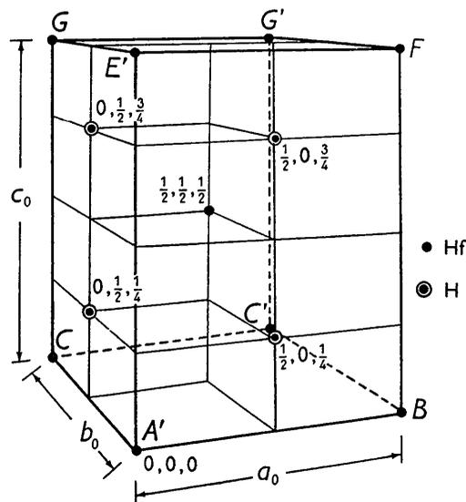
Fig. 1. Body-centered tetragonal unit cell of  $\text{HfH}_2$  structure.
