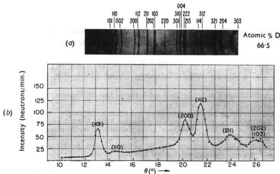
Fig. 2. (a) X-ray diffraction pattern of  $\text{HfD}_2$  (Co  $K\alpha$  radiation; camera diameter 114.6 mm.). (b) Low-angle portion of neutron diffraction pattern of  $\text{HfD}_2$ .
