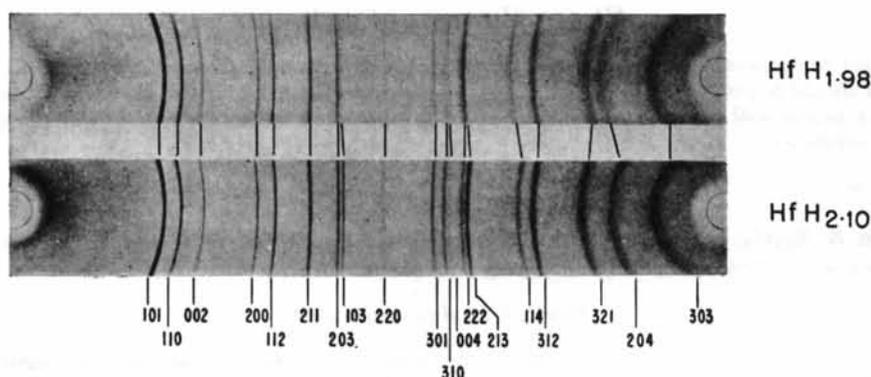
Fig. 3. X-ray diffraction pattern of hafnium dihydrides (Co  $K\alpha$  radiation; camera diameter 114.6 mm.).
